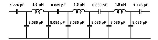
The first thing to notice is that it's ripe for embedding. The L and C values are close to the bottom of the range for consumer equipment and lower values can be embedded with higher yield, better reliability, and, of course, smaller footprint. To be an economical design, this whole thing needs to come in no larger than a few mm<sup>2</sup>.
